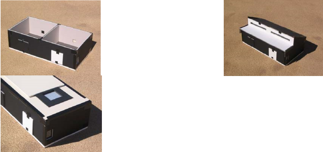
Fig. 3 Physical model photographs: base case with no roof, 2 ft glazing clerestory, and 7% glazing skylight cases.
