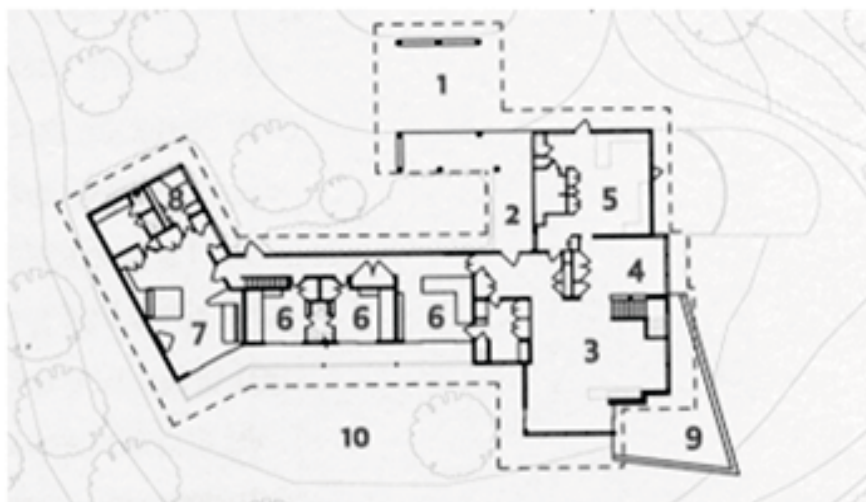
Figure 5: Floor plan of the Liljestrand House: 1 carport, 2 entry, 3 living room, 4 dining room, 5 kitchen, 6 bedrooms, 7 master bedroom, 8 study, 9 deck; in the ground floor, a family room below 3, and a recreational room below 6s open to 10 lawn. (Sakamoto, Britton, and Murphy 2007)
