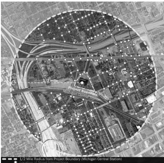
Figure 10: Neighborhood Pattern and Design (NPD) - An intersection count was conducted within a 1/2 mile radius of Michigan Central Station in Southwest Detroit. The results revealed a total of 165 intersections, surpassing the minimum requirement of 140. (Studio[Ci], 2011)
