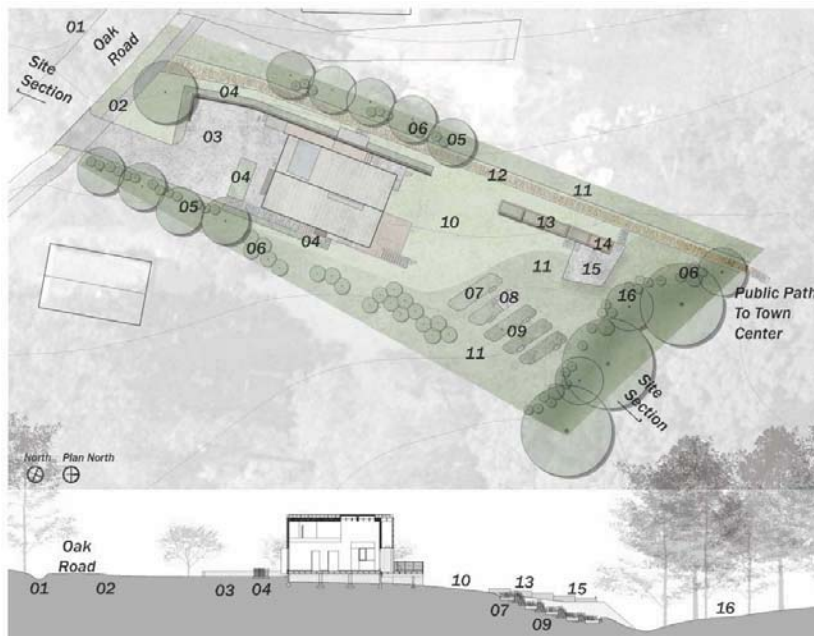
Figure 2: Site Plan and Section. 01 Existing Swale; 02 Sidewalk; 03 Parking Court/Site of Original Demolished Home; 04 Perennial Bed; 05 Small Native Trees; 06 Native Shrubs; 07 Greywater Treatment Bed; 08 Forebay/Rainwater Inlet; 09 Rainwater Infiltration Beds; 10 Drought Tolerant Turf; 11 Native Grass Meadow; 12 Crab Orchard Stone Community Path; 13 Raised Vegetable Beds; 14 Irrigation Cistern Enclosure/Hand Pump; 15 Gravel Patio and Fire Pit; 16 Existing Swale/Forest.
