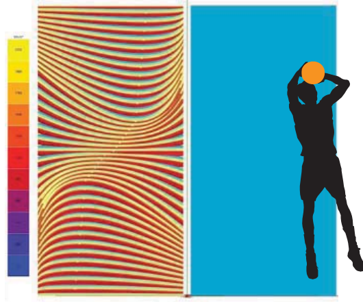
Figure 13: Color-coded comparison of amount of total annual incident radiation of proposed panel (left) to a flat panel (right). Source: (Author 2013)
