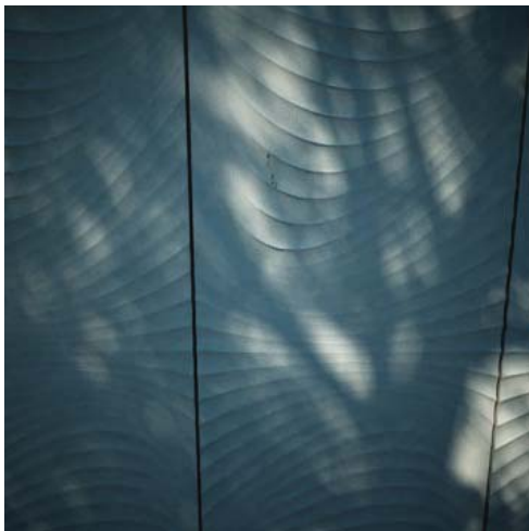
Figure 14: Close-up of proposed photocatalytic concrete panel. Source: (Author 2013)
