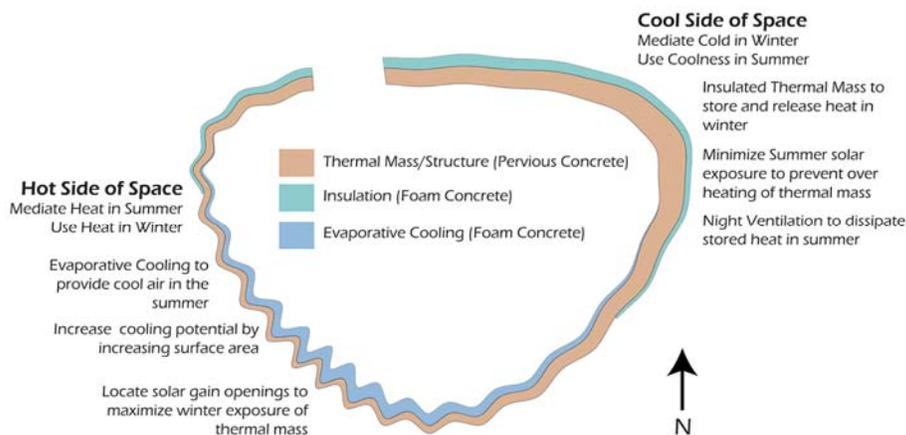
**Figure 3:** Schematic plan showing placement of foam and pervious concrete. Source: (Johnson 2012)
