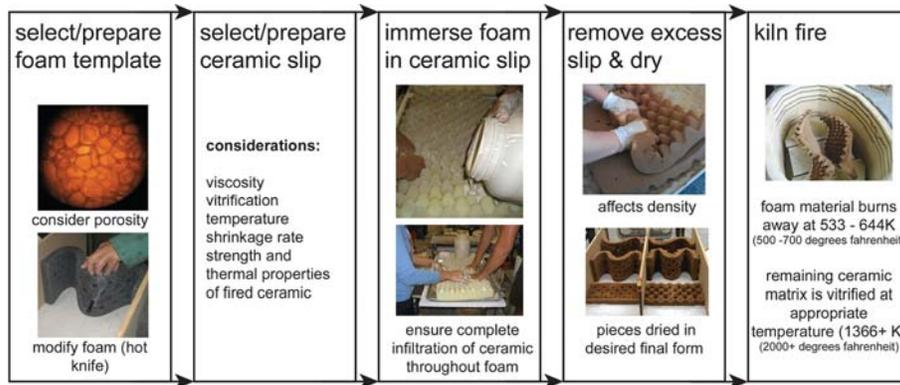
**Figure 1:** Process of Replication to make cellular ceramic. Source: (Johnson 2012)
