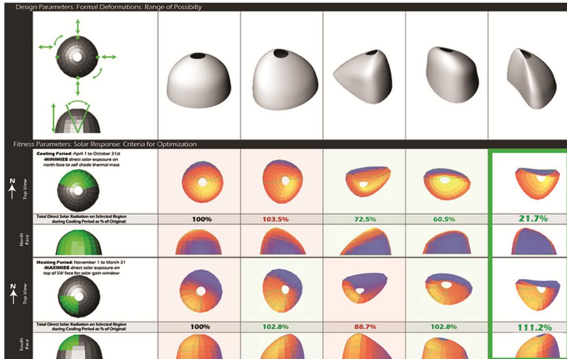
**Figure 4:** Results of digital optimization process relating to solar radiation. Source: (Johnson 2012)
