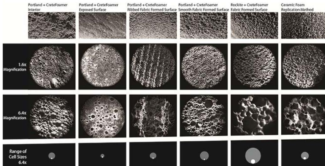
**Figure 2:** Microscopic Images of various samples using various material compositions and forming techniques. Source: (Johnson 2012)
