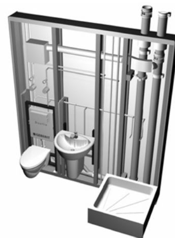
Figure 10. Digital representation of the core wall by MIT House_n and Bensonwood Homes. Source: (Open Prototype Initiative 2006)
