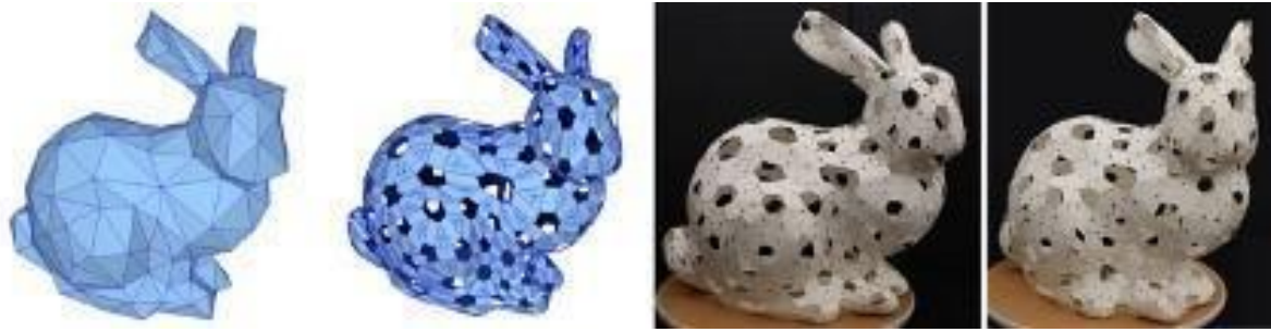
Figure 9. An example demonstrating the power of our method to construct any shape with similar panels.
